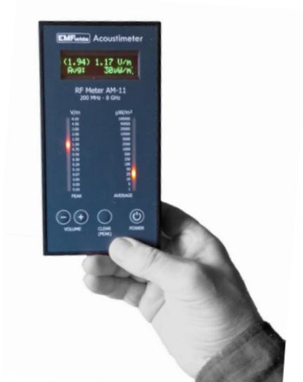
Ideally hold the meter as shown in the picture. Try to keep the Acoustimeter at least 30cm away from your body when taking readings. Keep your hands towards the bottom of the instrument.
